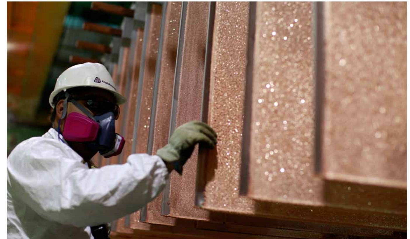
Yuri Varas in the processing plant at the leaching stage - Inspecting copper anodes
