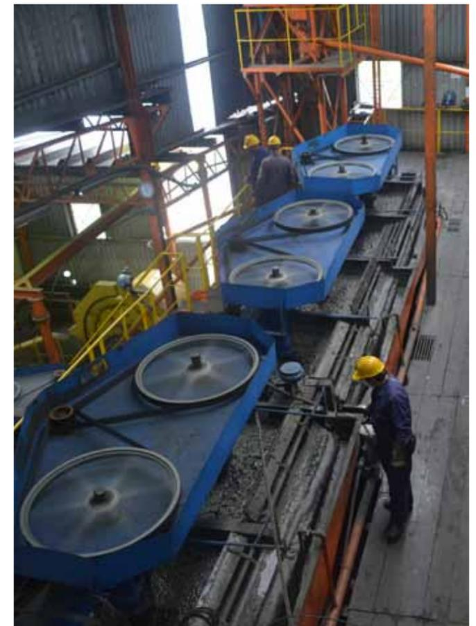
El Roble Mine, Flotation Circuit
