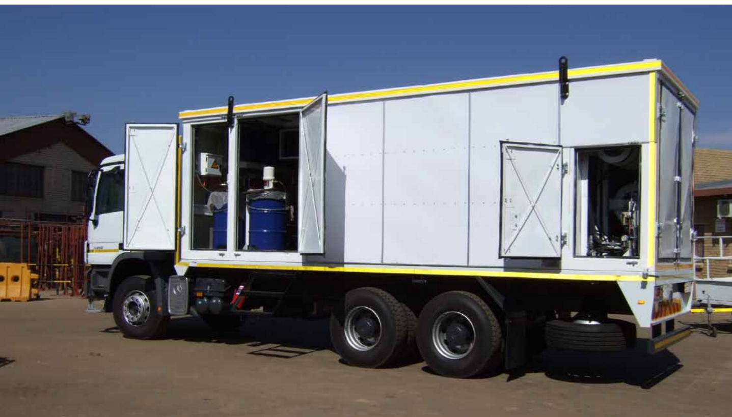
Lube service unit
