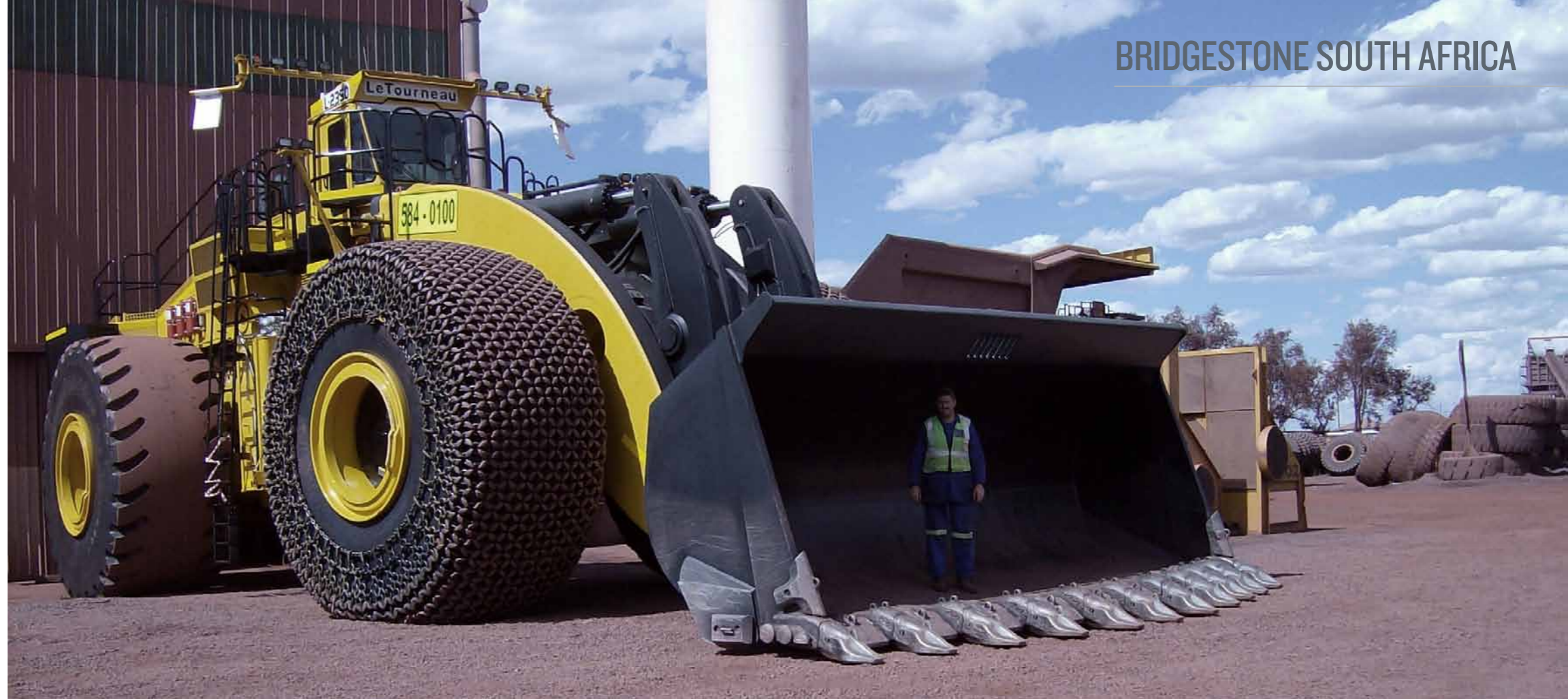
Le Tournou L2450 front end loader at Sishen Mine
