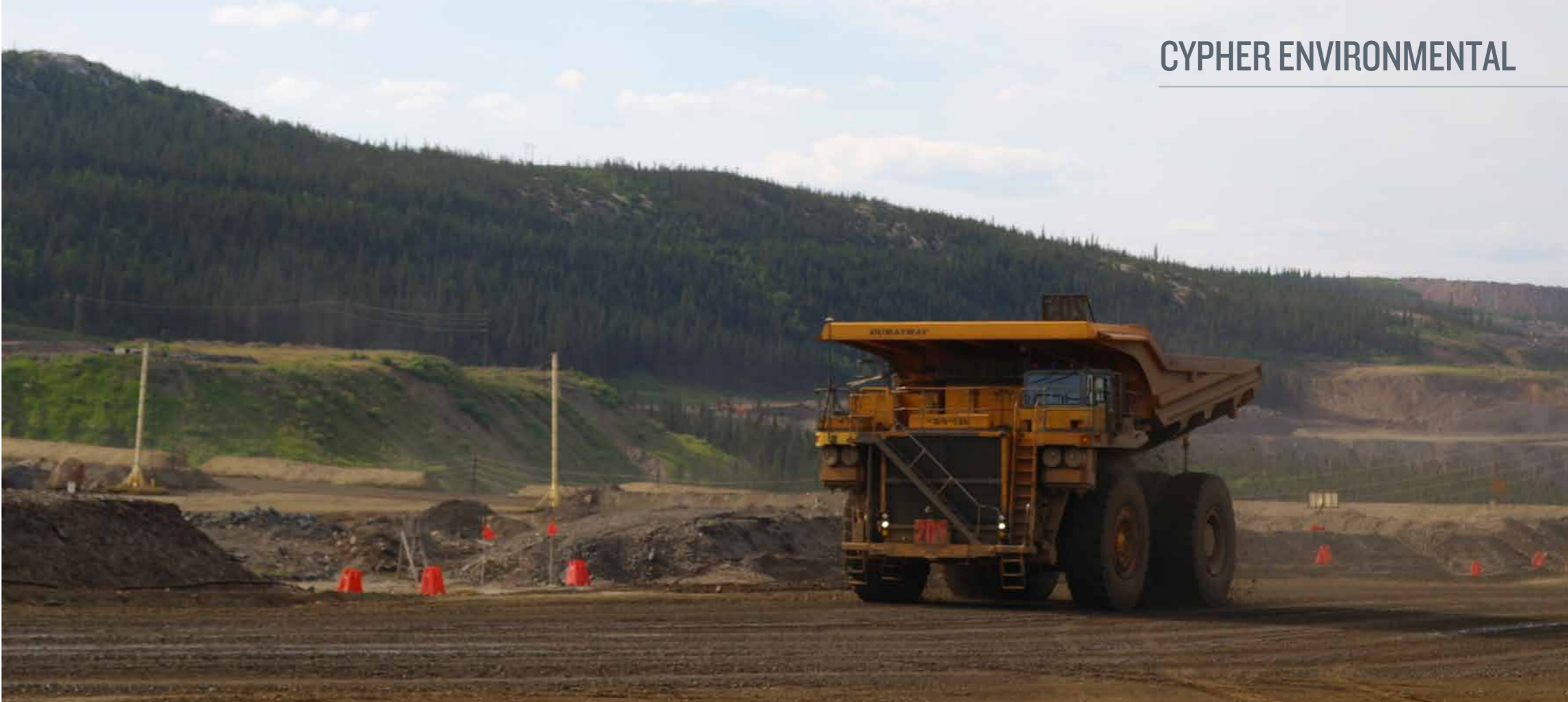
Empty haul truck traveling on the same Dust Stop treated road at a mine site in Eastern Canada
