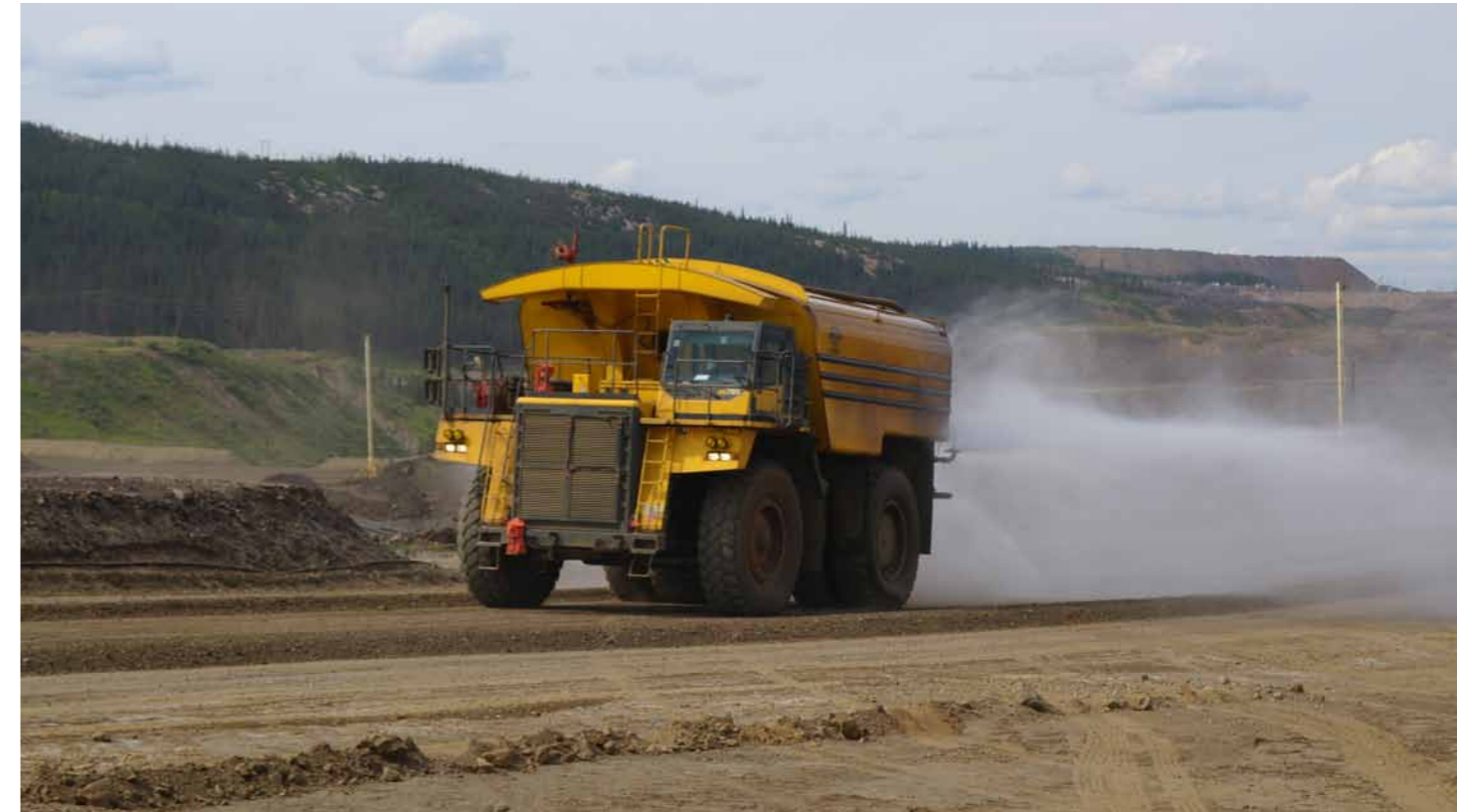
Dust Stop being applied to the road surface
