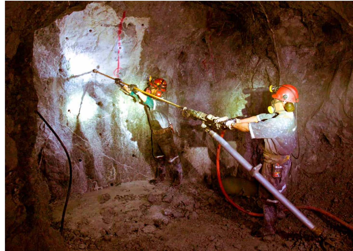
Jackleg drilling of the stope face in Guanajuato
