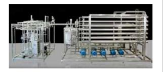
causes the feed liquid in circulation to scour the surface of the membranes creating a constant cleaning effect with minimized chemical cleaning. Modular design allows for any flow rate with capacities which can be increased at a later stage by adding more modules.
