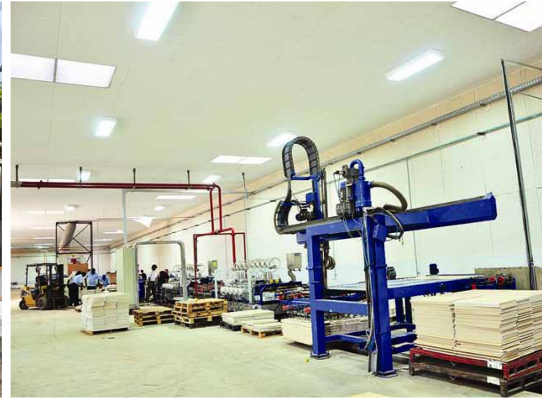
Rectification and chamfering of tiles
