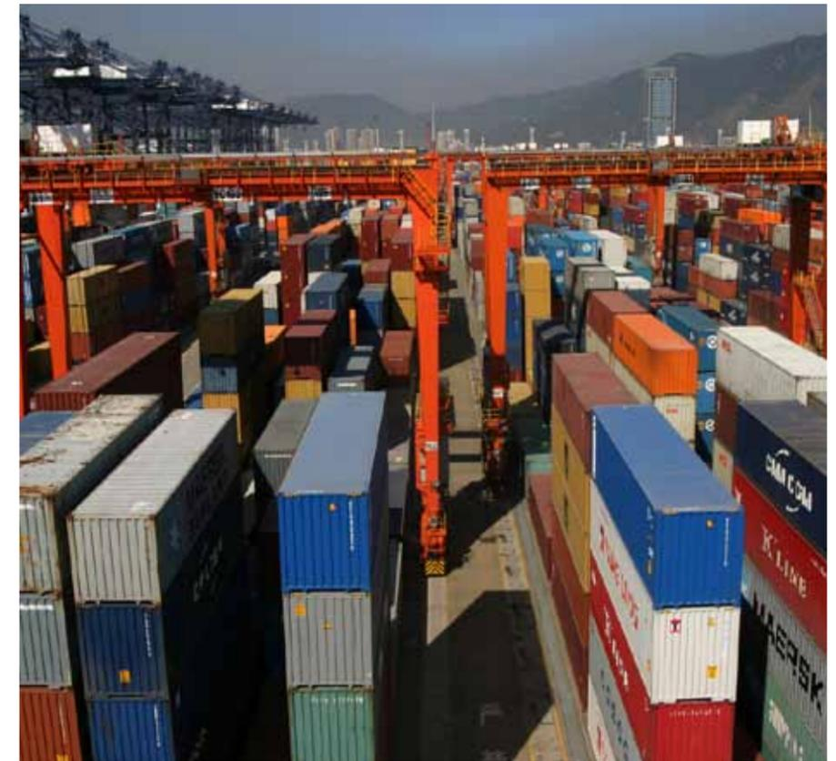
reduce port emissions and save fuel through the use of electric power rubber-tyre gantry cranes (RTGCs). Today we have 150 of these RTGCs in use, as well as a further 19 hybrid RTGCs, which run both on both electricity and diesel, helping to reduce fuel and carbon emissions by 40 percent.”
