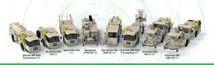
Normet SmartDrive is a modular battery electric vehicle (BEV) architecture designed to optimize energy consumption and performance in underground mining and tunnelling applications. Normet SmartDrive equipment enables higher productivity, lower operating costs and most importantly - zero local emissions. Ease of use and carefully engineered controls ensure safe and pleasant operation. High power motors reduce tramming time and recover energy in downhill driving.
