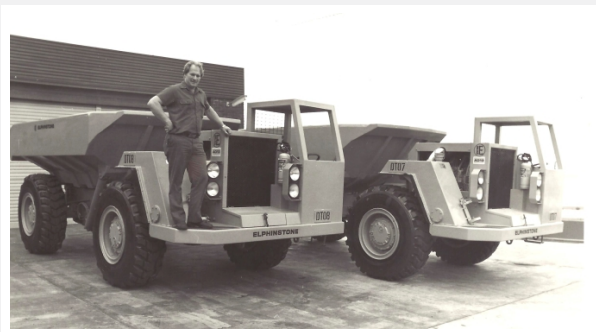
Elphinstone's first purpose-built underground dump trucks were the AD13 (pictured), and Ad17.
